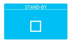
Press the +/- keys to check or uncheck, confirm and exit with **OK.** Press **ON/OFF** to exit without saving and return to the main screen.
