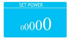
Using the +/- keys it is possible to select the desired power from 1 to 5; press the OK button to confirm the power.
